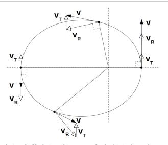
Fig. 1 The velocity of a Keplerian orbiter  $\mathbf{v}$  on a fixed orbit is always the sum of a uniform rotation velocity  $\mathbf{v}_R$ , perpendicular to the vector radius, and a uniform translation velocity  $\mathbf{v}_T$ , which direction is always perpendicular to the main axis of the conic. Both are coplanar and have a constant norm all along the trajectory.
